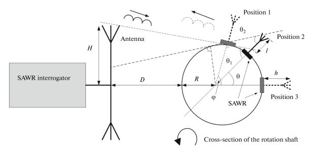
Fig. 1. The illustration of SAW rotation speed measurement system.
